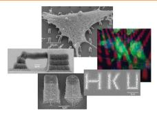
Multiphoton-based free-writing of 3D complex protein microstructures and micropatterns, with sub-micrometer features and controllability over voxel dimension, morphology, and porosity, is reported. Protein micropillar array presents a simple "write-and-seed" platform for cell niche studies. Fibroblasts attach to, grow on, express adhesion molecules and deposit extracellular matrices on these arrays without matrix coating.
