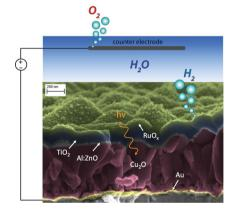
Ruthenium oxide on cuprous oxide photocathodes enhanced by a built-in p-n junction yields an active catalyst for hydrogen generation from water and unprecedented 94% stability over 8 h of light chopping chronoamperometry at 0 V vs. the reversible hydrogen electrode. The photocurrents obtained would correspond to greater than 6% solarto-hydrogen efficiency in a tandem cell configuration.
