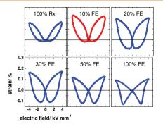
Incipient piezoceramics are featured by giant strain of ≈0.4%. However, this giant strain is only realized at relatively large electric field (>4 KV mm<sup>-1</sup>) with a significant strain hysteresis. Here, many of the challenges the incipient piezoceramics face can be overcome by relaxor/ferroelectric composite approach.
